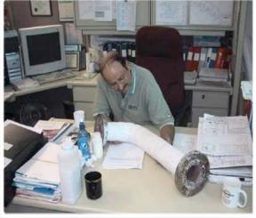
Leaking Pipe, rebuilt with **CerarMix**<sup>™</sup> passed a 24 hour steam test at 150psi
