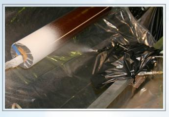
**CerarMix**<sup>™</sup> applied by patented spray system to pipe mandrel creates monolithic void-free liner with superior abrasion resistance.
