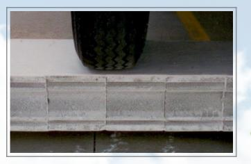
The CerarMix<sup>™</sup> coats six standard concrete blocks with no mortar or additional support. It withstands over 4000psi
